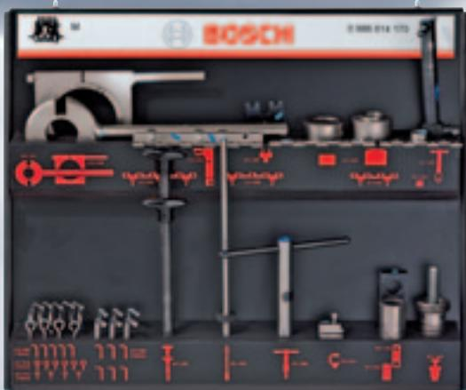
Repair of in-line fuel-injection pumps of model series PE(S) ..M.. with and without port-closing sensor system (FBG system), **without** controller, atmospheric-pressure-dependent full-load stop (ADA) and timing device
