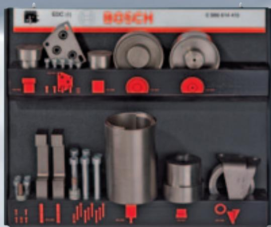
**Tool set** for the repair of actuator mechanisms (RE actuator mechanisms) of electronic controllers for the in-line fuel-injection pumps of sizes R, M
