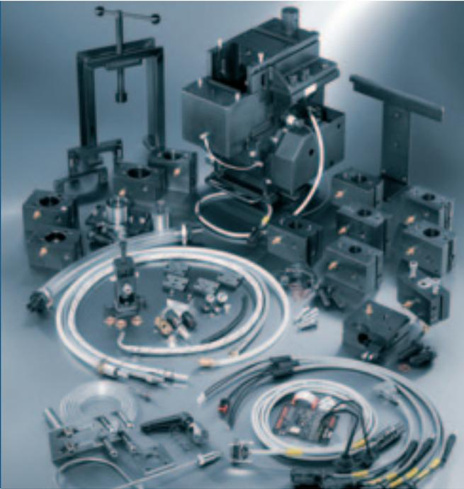
The basis for testing Unit Injector and Unit Pump systems is the complete package. It contains the Cambox and 12 adapters required for testing UI and UP systems from Bosch.
