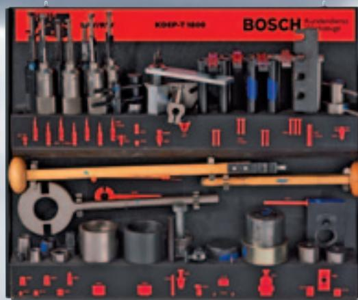
Repair of in-line fuel-injection pumps of model series PE(S) ..MW.. S1 (8 mm stroke) ..S100 (10 mm stroke) and ..S1500, **without** controller, charge-pressure-dependent full-load stop (LDA) and timing device
